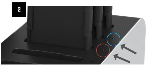
When case is inserted correctly, an LED indicator light will illuminate.
