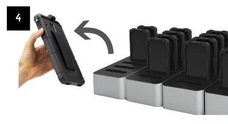
To remove, simply pull up on Flex case. Magnetic charger will detach automatically.
